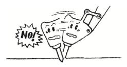
Don't use the chisel to move rock or use as a lever to pry rock. It will damage through bolts, chisel, bush, etc.
